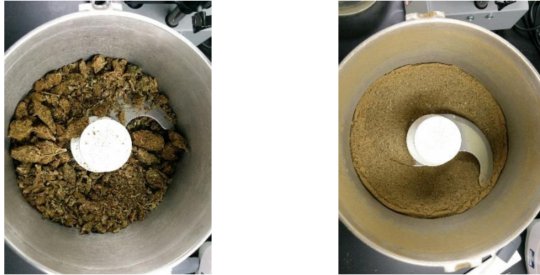
Figure 1. Cannabis sample before (left) and after (right) homogenization with dry ice.
