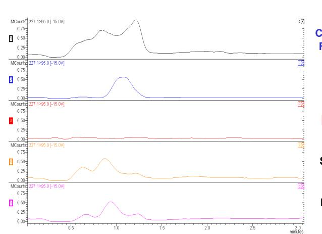
Figure 2: LCMS responses for Tween 20 in elution fractions of several extraction devices including Plexa DAS.
