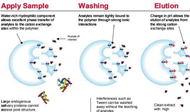
Figure 1: The three stages of extraction and key functional properties observed when using Plexa DAS.
