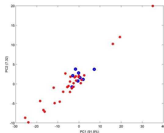
**Figure 3.** PCA scores plot of authentic (blue) and counterfeit (red) vodkas applied to the peak ratios with respect to ethanol.
