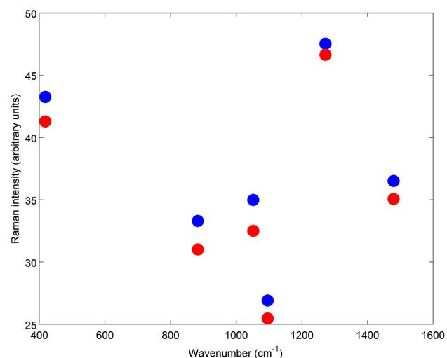
**Figure 2.** Average alcohol content of authentic (blue) and counterfeit (red) calculated from the six principal ethanol peaks at 418, 883, 1052, 1096, 1272 and 1450  $\text{cm}^{-1}$  respectively.
