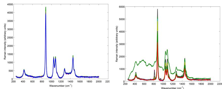
**Figure 1.** Raman spectra of authentic and counterfeit vodka samples.
