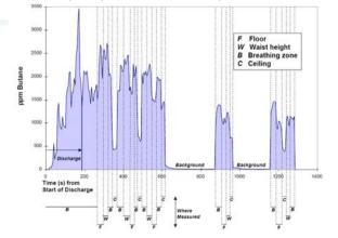
Figure 4. Vapour analyser reading (butane) for a 170 ml anti-perspirant deodorant fully discharged in a small room.
